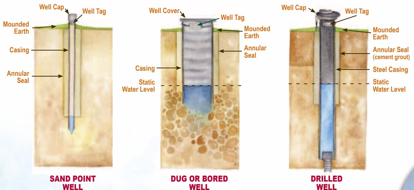
The most common types of wells constructed in Ontario are the Sand point (Jetted), Dug or Bored, and Drilled. A properly constructed well is tightly sealed to prevent anything but groundwater from entering it. It's critical to seal the well from surface runoff as a single gram of fecal matter can have up to 1 billion bacteria.
