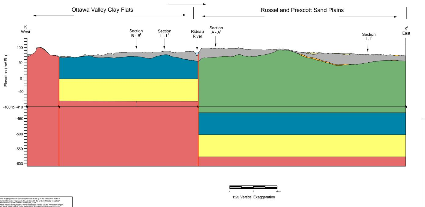
Legend — Fault **Formation** Surface Water Sand (Quaternary Deposits) Gravel (Quaternary Deposits) Clay (Quaternary Deposits) Ottawa Formation (Shale/Limestone/Sandstone) Oxford/March (Dolostone/Limestone)
